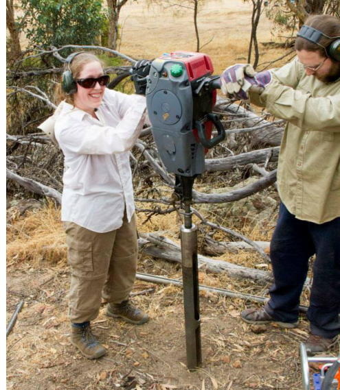
Valerie Miller drilling soil cores at University of Western Australia Future Farm to assess chemical and biological properties of soil for critical zone research. Photo by David Huber.
